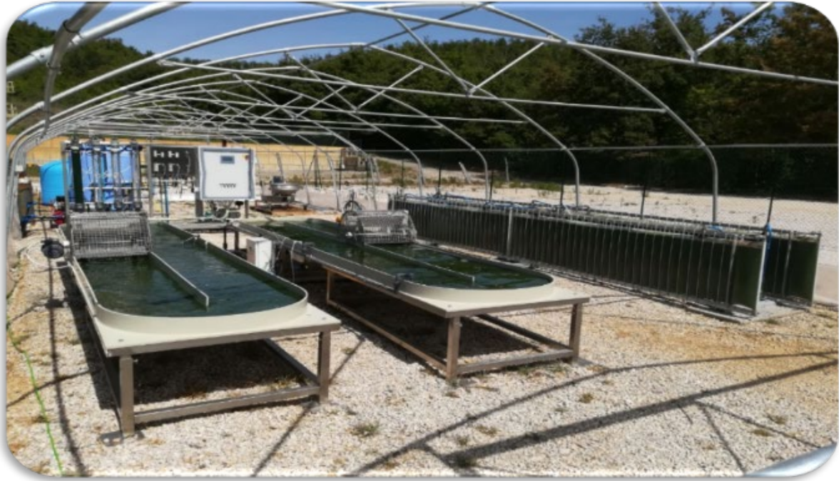
Figure 12.7: Spirulina pilot plant at Chiusdino power plant
