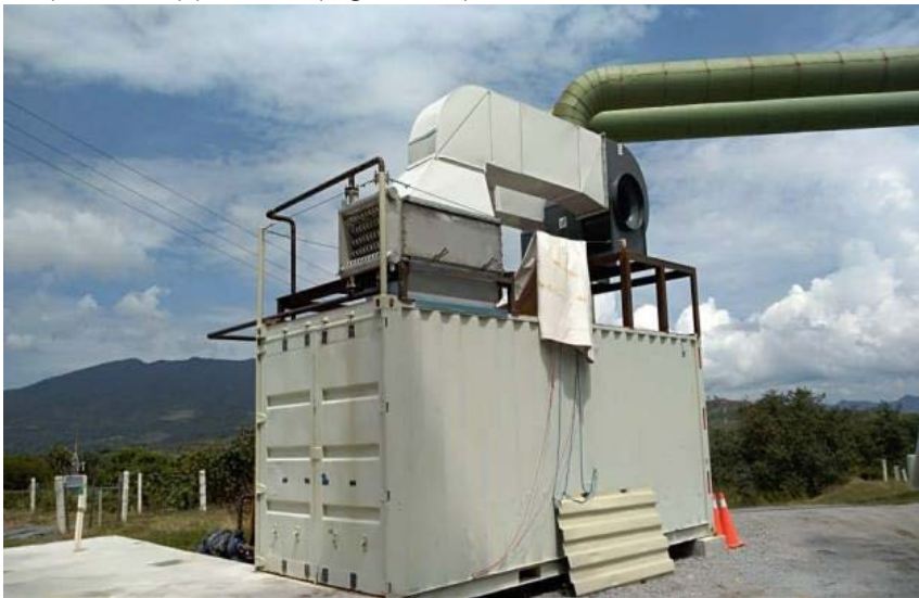
Figure 3-2 Food Dehydrator model DGA200 at the Domo San Pedro Field Mexico. Photo courtesy CeMIEGeo 2017 update report to the IEA Geothermal Daejeon Geothermal Workshop 9 November 2018.
